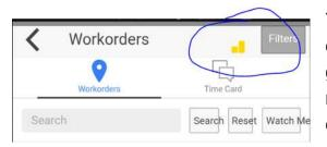
Yellow bars indicate that the signal is weak and not optimal to submit a job. Moving a few steps will usually give you the green bars as wireless signal does not radiate in a uniform pattern from the tower but can be obstructed by many obstacles.
